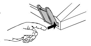
Figure 4: Ejecting the MOBILINK from the Slot
